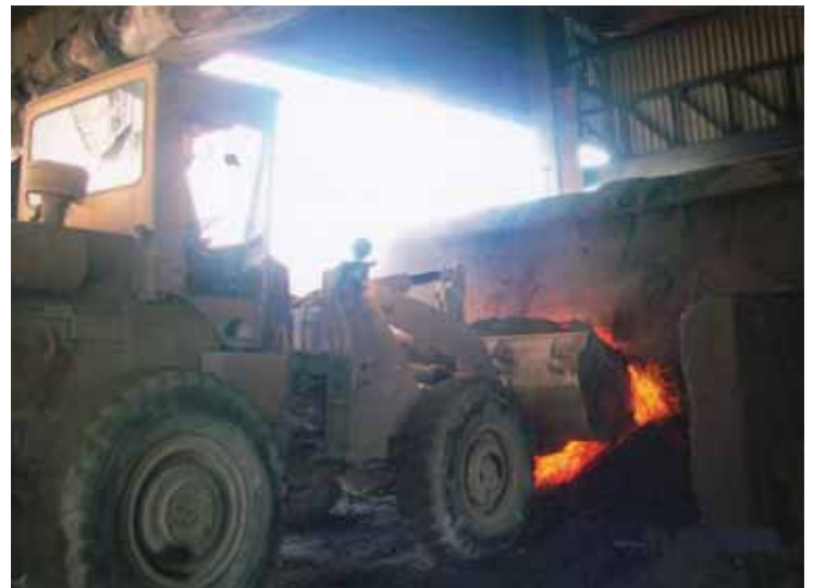
LOADER IN OPERATION UNDER THE CONVERTERS FOR CLEARING OF SPILLAGE AT JINDAL STEEL WORKS LTD. (JSW)
